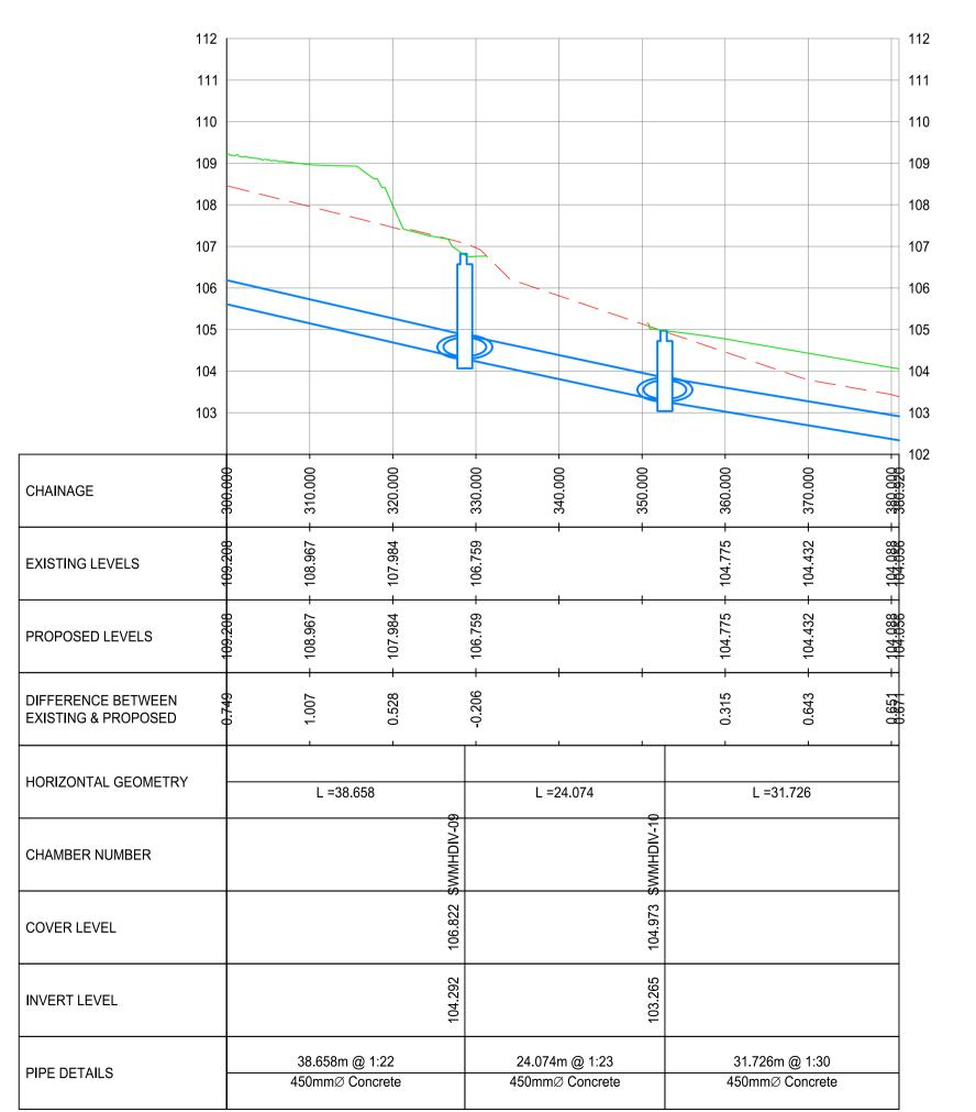
STORMWATER DIVERSION (1) SCALE: H 1:500,V 1:100. DATUM: 102.000
